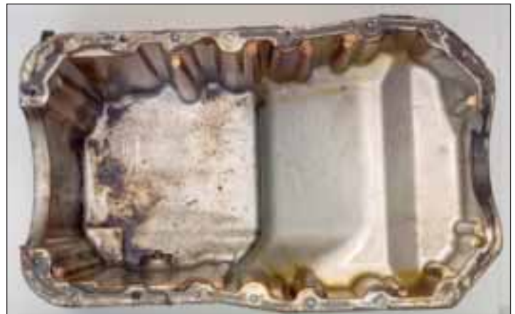
The inside of the engine oil pan was very clean. There were no sludge deposits found in the bottom of the pan.
