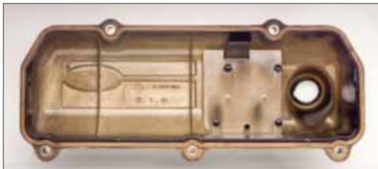
The inside of the valve cover was very clean. There were no sludge or heavy varnish deposits present. Note that you can still read the manufacturer’s markings.
